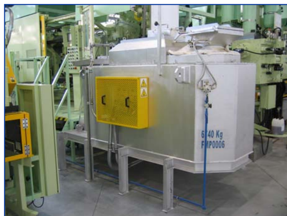
IMAE Holding Furnace next to High Pressure casting machine.
