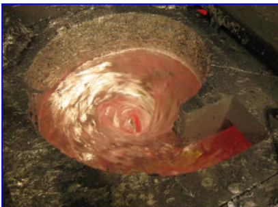
Ingot bundles or sows melting in the dry hearth
