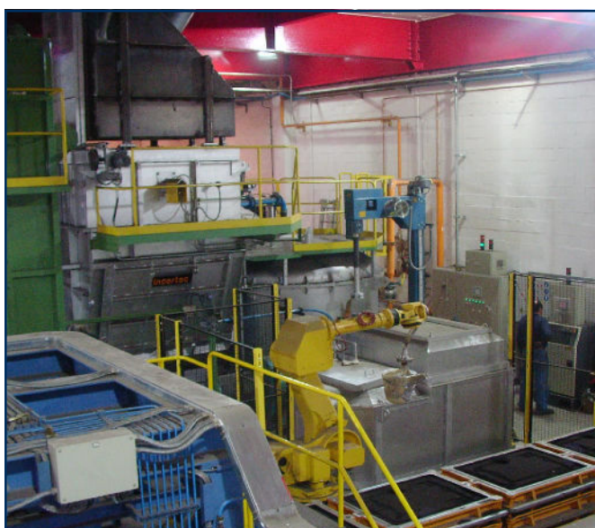
MELHOLDER® InLine 2000 kg/hr on gravity sand mould casting line
