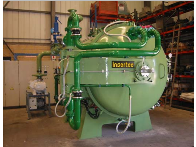
Horizontal-loaded Vacuum Furnace for Hardening under N 2 atmosphere up to 10 bar.
