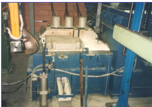
Degassing rotor, vertical heaters and pneumatic open well lid
