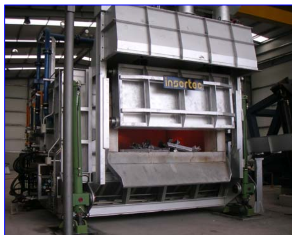
Detail of main doors with dry pre-cast shape frames
