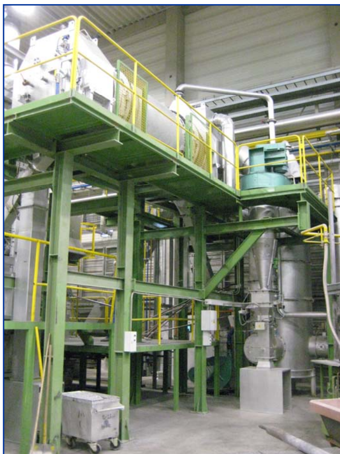
IDEX-1000 with Vertical Afterburner Chamber
