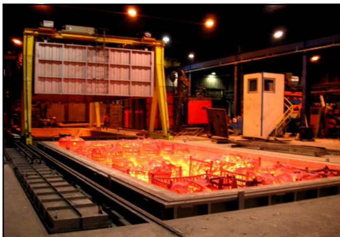
Travelling Bell type Chamber Furnace provided with two load-unload bases.
