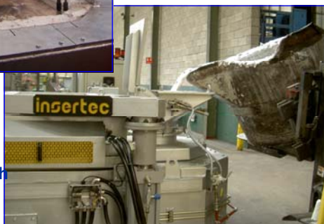
Charging hopper with pneumatic lid
