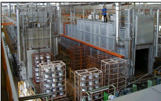
General view of T6 Heat Treatment Installation based on "U" type arrangement.
