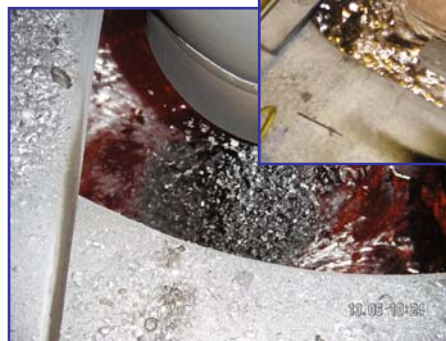
Sink Vortex Chamber with Chips entrainment
