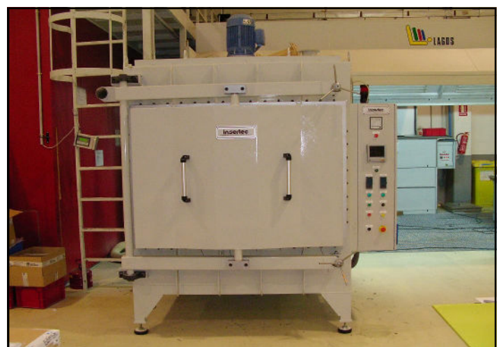
Chamber type Recirculation Furnace provided with hinged front door.
