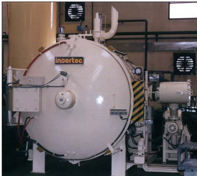
Horizontal-loaded Vacuum Furnace for Annealing and Tempering.
