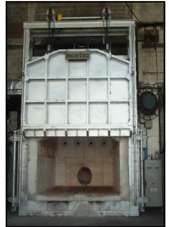
Chamber Furnaces provided with sliding front door.
