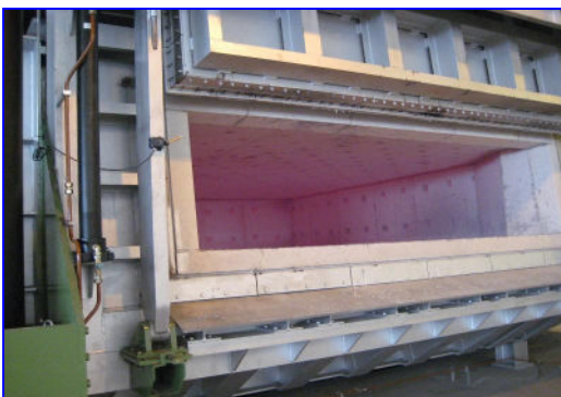
Main Door with SIFCA precast frame
