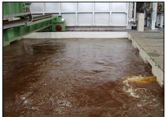
Quenching Tank (water, oil or polymer).
