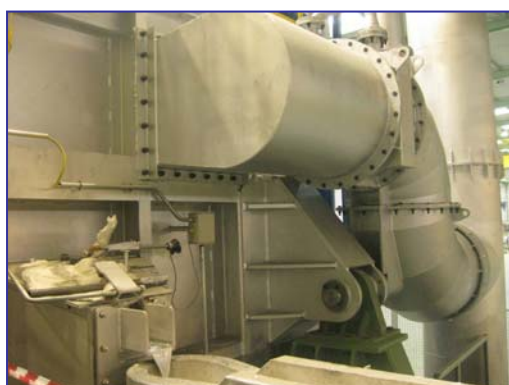
Detail of the pouring spout aligned with the tilting axis and rotary exhaust exit
