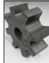
Furnace Lining made by Precast-Shapes
