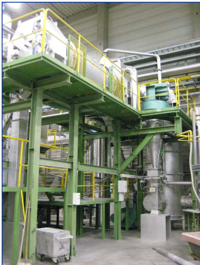
IDEX-1000 with Vertical Afterburner Chamber
