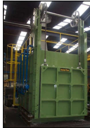
Chamber Furnaces provided with sliding front door.
