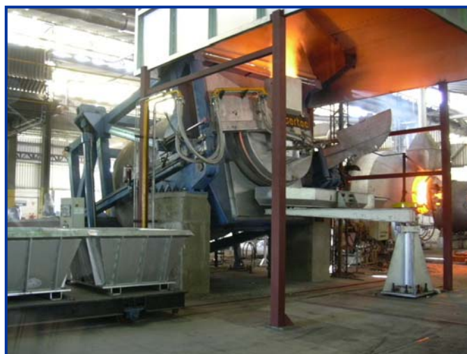
Tilting Rotary Furnace FARB-16
