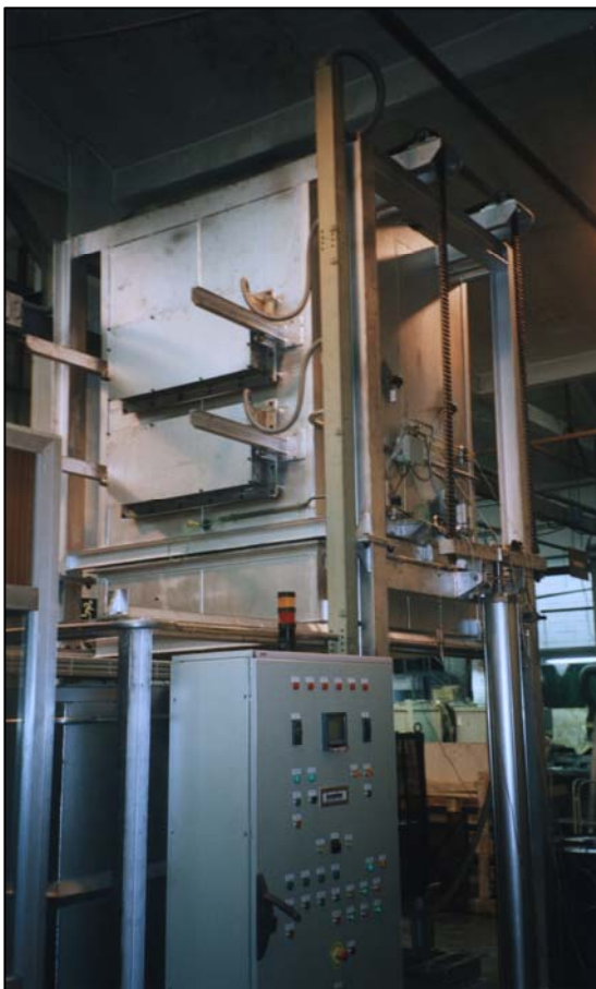
Rear view illustrating electric control panel and electric heating system.
