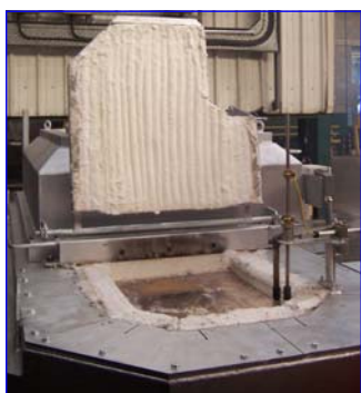
Ladling well with T/C and level sensor
