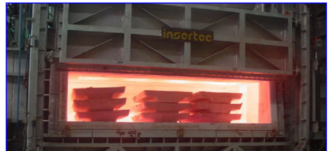
Ingot bundles or sows melting in the dry hearth
