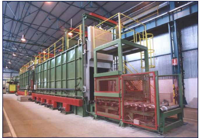
General view of T6 Heat Treatment Installation based on lineal arrangement.
