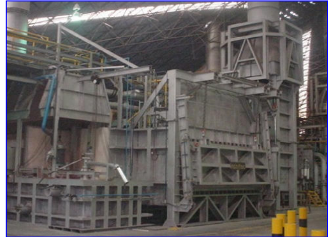
Stationary HIRARO Furnace 70 ton capacity & 8 ton/hr melting rate
