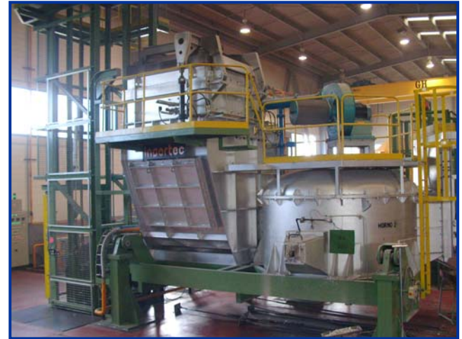
2 ton/hr Tilting Meltower General view
